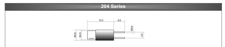
Dimensions in mm (Typical) Not to scale Colour dot on product sleeve denotes LED colour. Green dot on base indicates anode +ve termination.
